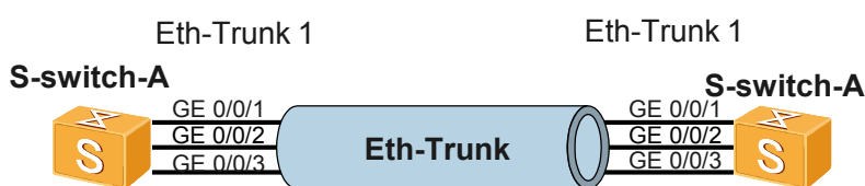
Figure 2-4 Networking diagram of link aggregation in manual load balancing mode
